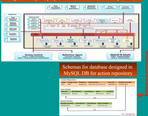
When the user approaches the PACS system to retrieve an image from the DI-r, the **Access Control** component captures the relevant information of the user required for making access control decisions.
